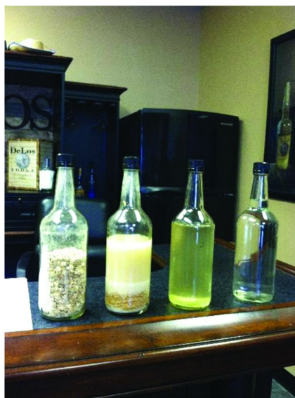
Figure 1. Stages of vodka separation. Bottles (l-r): wheat grains; yeast fermentation with gravity separation; filtration; first distillation giving vodka. (Photo credit: Diana Mason.)
